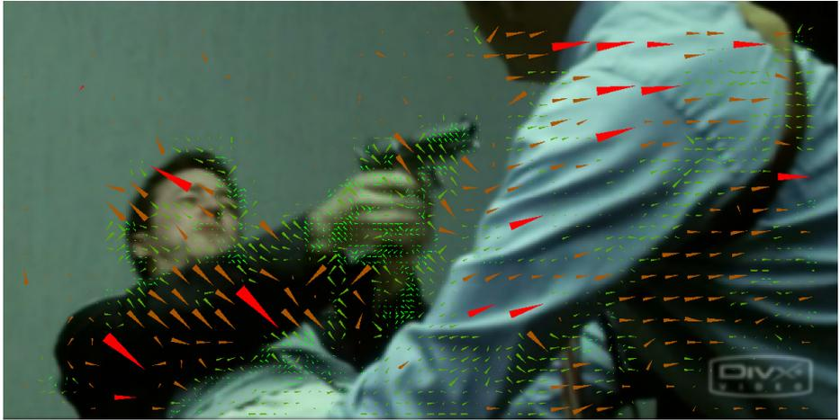
**Fig. 3.** VSBMA displacement vectors. Hotter colors indicate bigger blocks.
