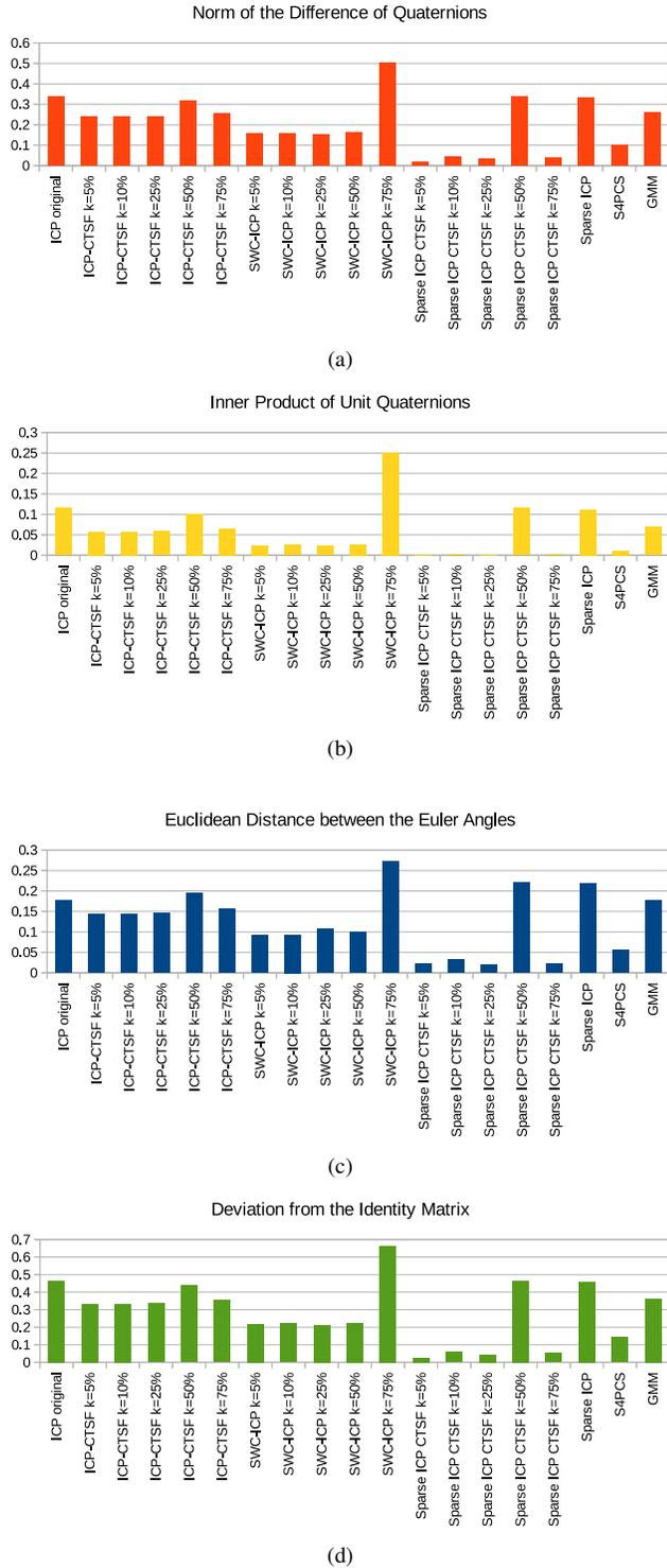
Fig. 7: Rotation error for the registration techniques (Trimming parameter  $\tau = 0$ ), for the case  $45^\circ - 90^\circ$ , computed using metric: (a)  $\phi_1$ . (b)  $\phi_3$ ; (c)  $\phi_4$ ; (d)  $\phi_5$ .
