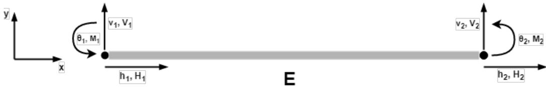
Figure 2.5: An element with three DOF per node and the forces exerted in each node.
